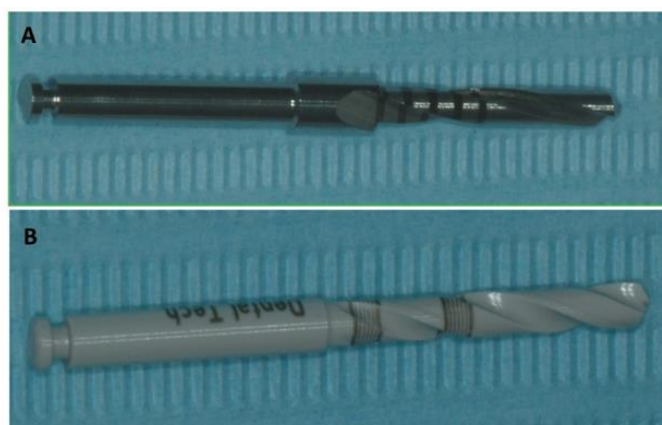
Figure 1. (A) Aspect of the stainless steel (SS) drill. (B) The aspect zirconia drill.
